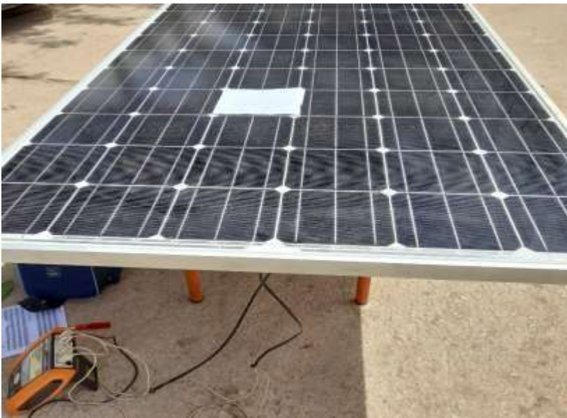
Figure 1. Mono module under test in partial shade. Source: results of my work
