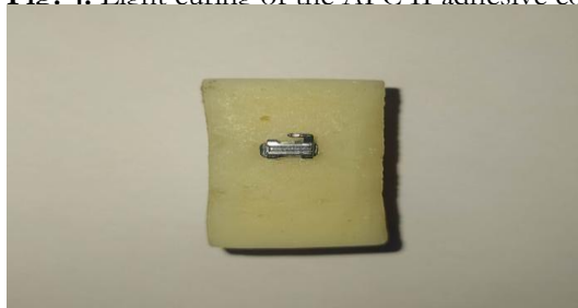
Fig. 5: Bracket bonded on the surface treated block ready for SBS testing.
