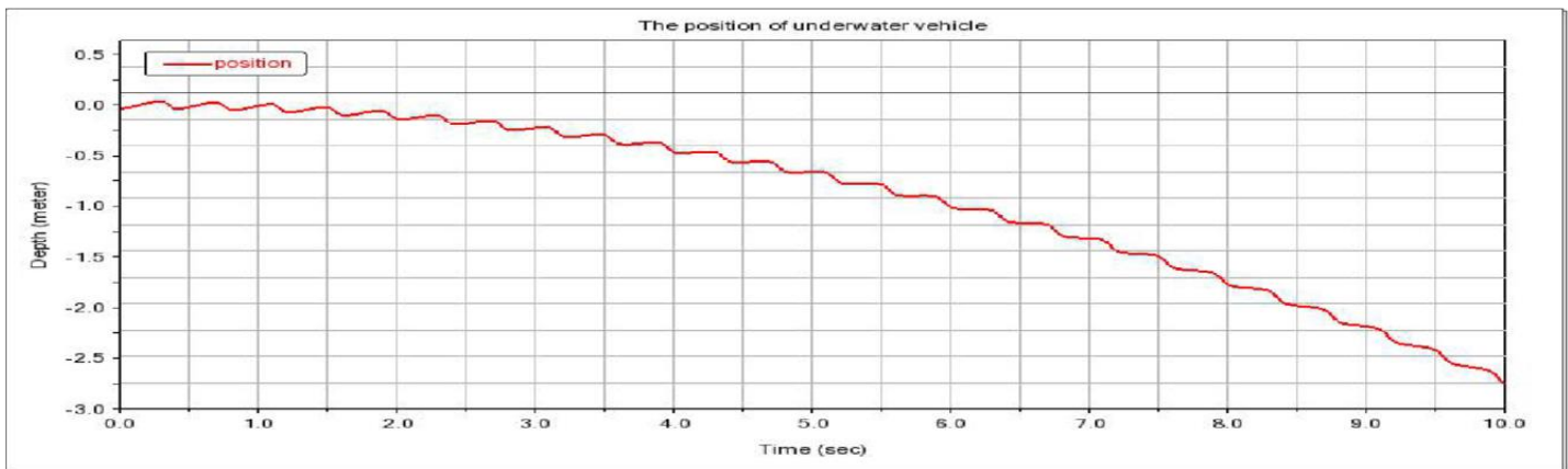
Figure 15: The change of the position of the center of mass in the first 10 seconds when harmonic motion.
