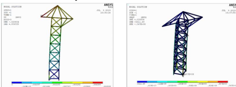
Figure 10: Z-direction displacement cloud. Figure 11: Equivalent force cloud.
