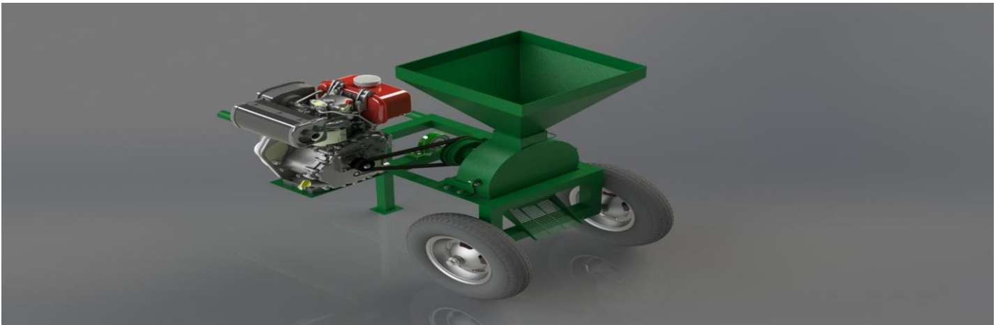
Figure 2.1: Three-dimensional model of the developed palm kernel nut cracking machine
